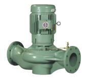
Taco 1900 Series In-Line pumps are compact, energy efficient and can be installed anywhere in the piping layout. The 1900 is designed to be self supported by the system piping (requiring no additional "strapping" or external support) and can be mounted horizontally or vertically. Permanently sealed grease lubricated ball bearings in the motor make the 1900 Series pump virtually maintenance free.
